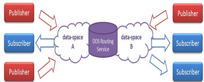
Fig 2.3 The DDS-RS transparently bridges DDS domains
